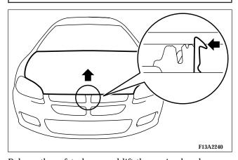
Release the safety lever and lift the engine hood.
